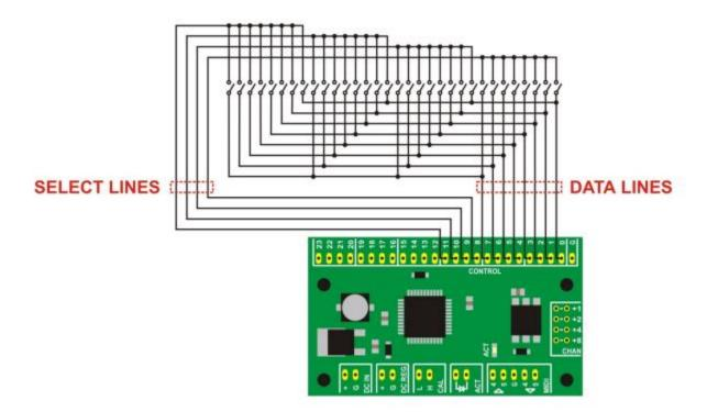
Between the CPU's switching matrix scheme and its ability to read encoder inputs, all of the user interface hardware is able to be handled by only 4 CPU's, all run serially together to send a single MIDI signal to the Raspberry Pi's for decoding and synthesis.
