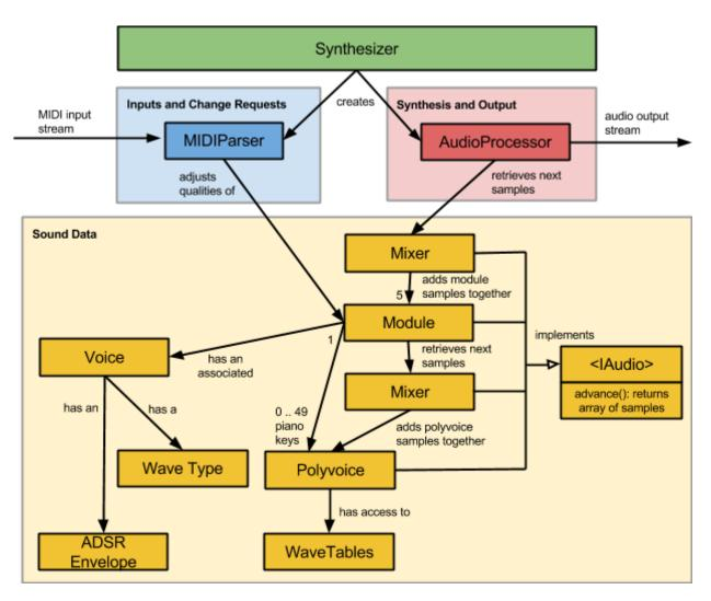
The diagram above shows a more detailed view of the software design inside the "Parsing and Sound Generation" module pictured in the System Design Diagram. It is important to note that the input of this module doesn't change whether the songbox is attached or not. There are three main components to this design: Inputs and Change Requests, Sound Data, and Synthesis and Output.
